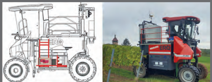
Fig. 3: Phenoliner: modified grape harvester; used to develop methods in vineyards for phenotyping and precision viticulture.
